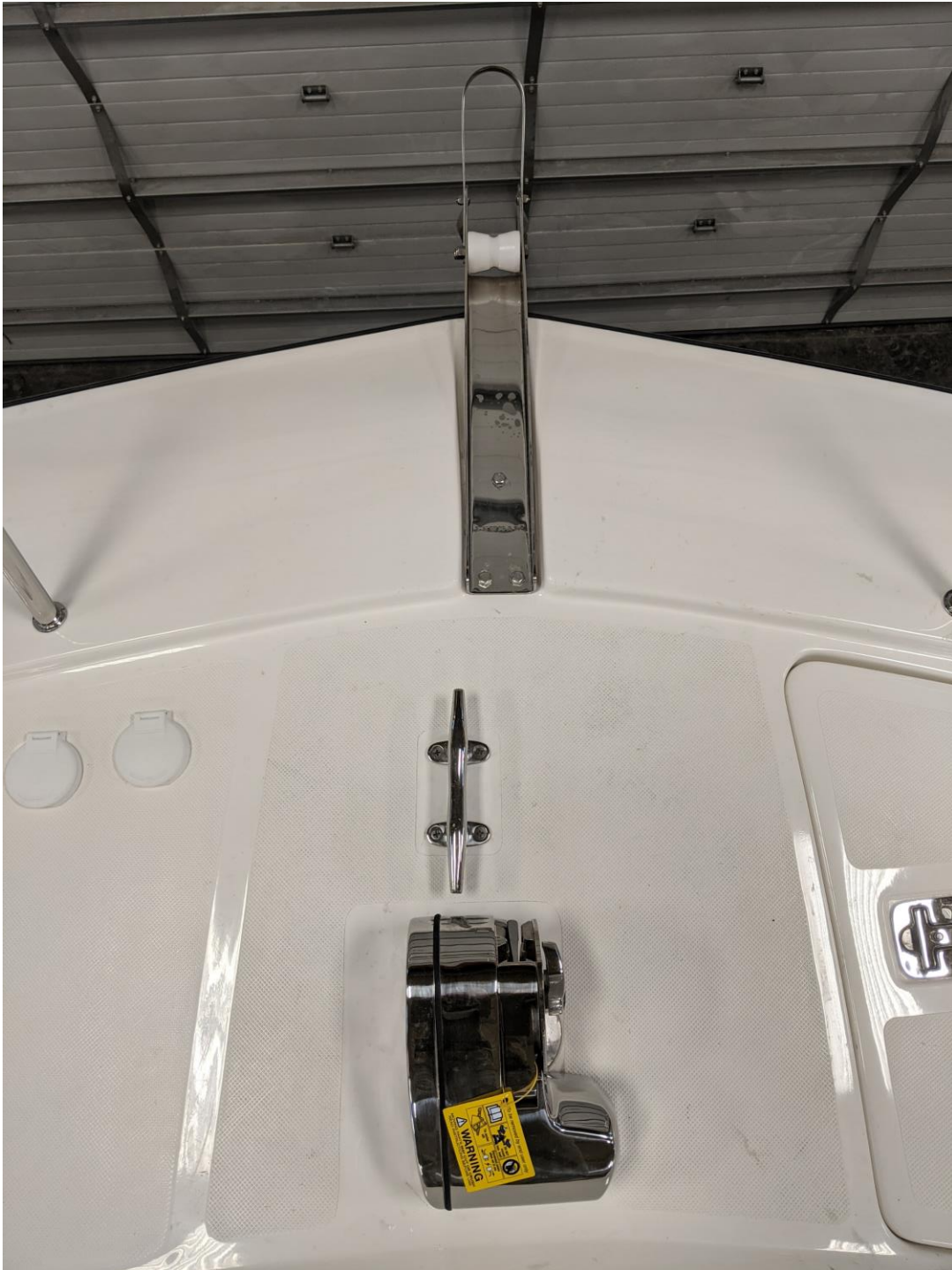
WINDLESS WITH CLEAT AND ROLLER (Be sure to add bungee or snubber to secure)
