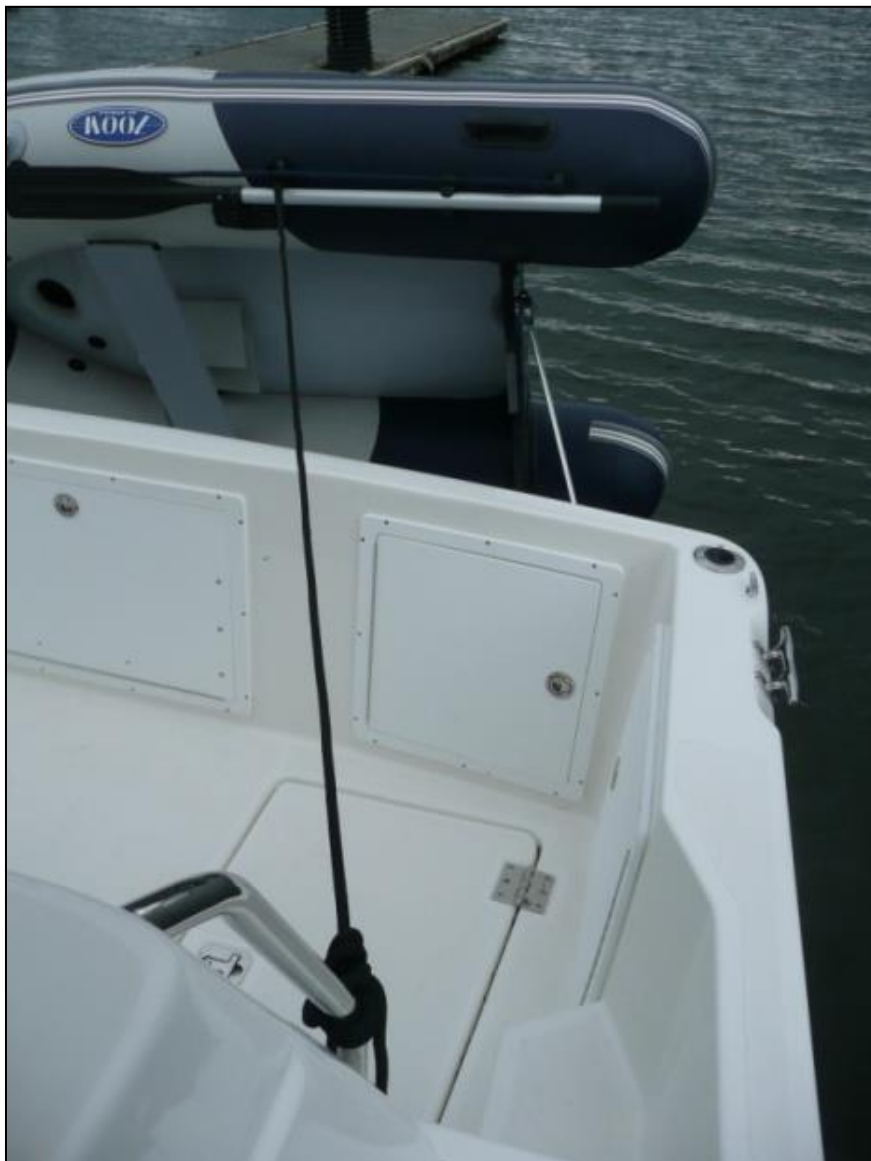
Tender Snubber Ling: used for medium range towing to take wind buffeting out. For long hauls it is best to deflate the tender. The line is also used to help with lower/raise tender.
