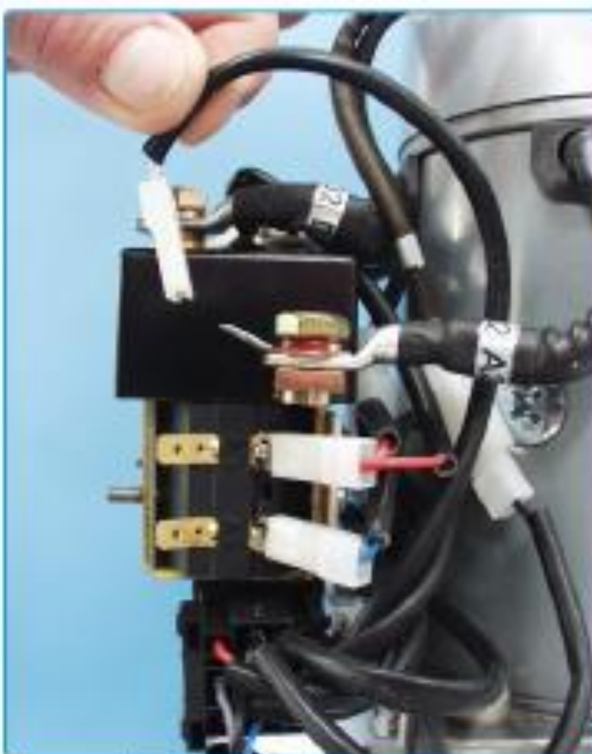
Disconnecting white IPC sensor wire
