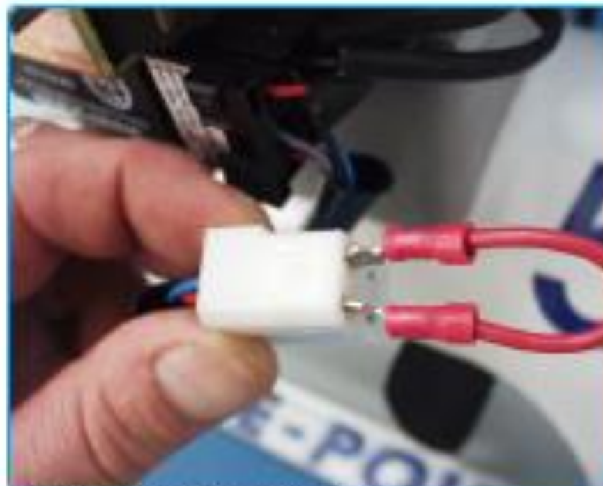
Jumping red to blue on motor pigtail
