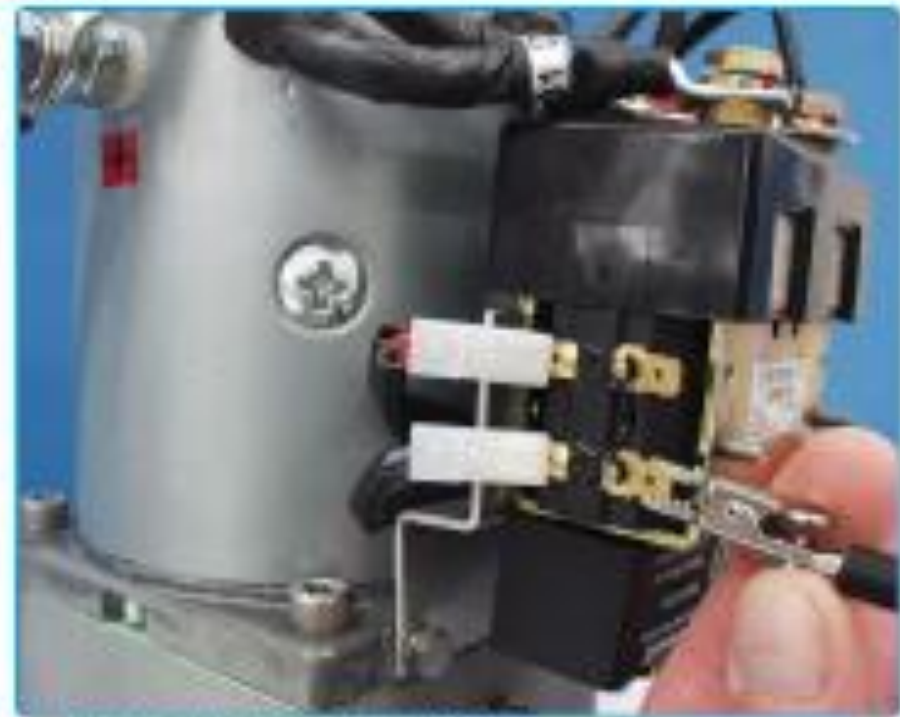
Jumping ground to grey on D1 coil
