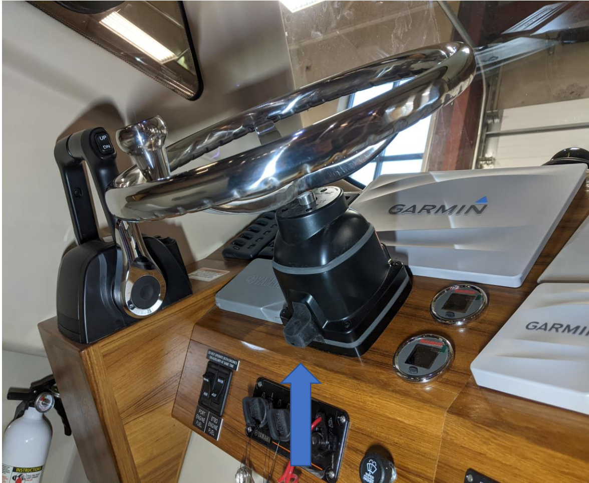
The Tilt Helm lever is located under the steering wheel.
