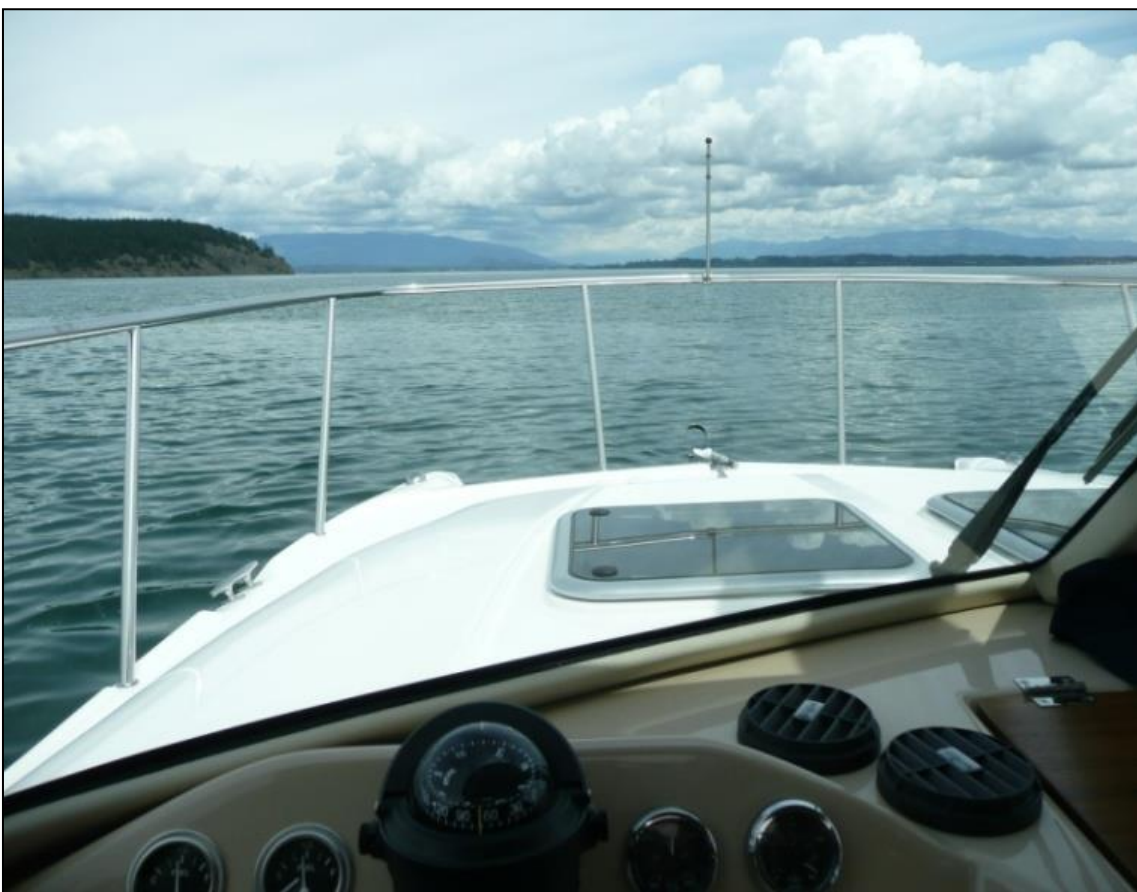
Running attitude, 16 Kts, tabs down.
