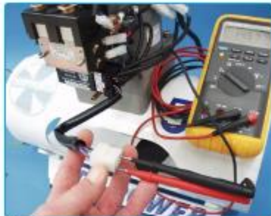
Checking voltage on motor harness
