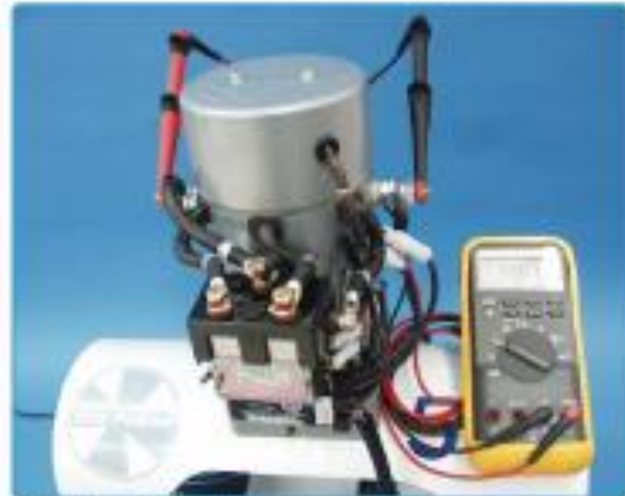
Checking voltage at thruster
