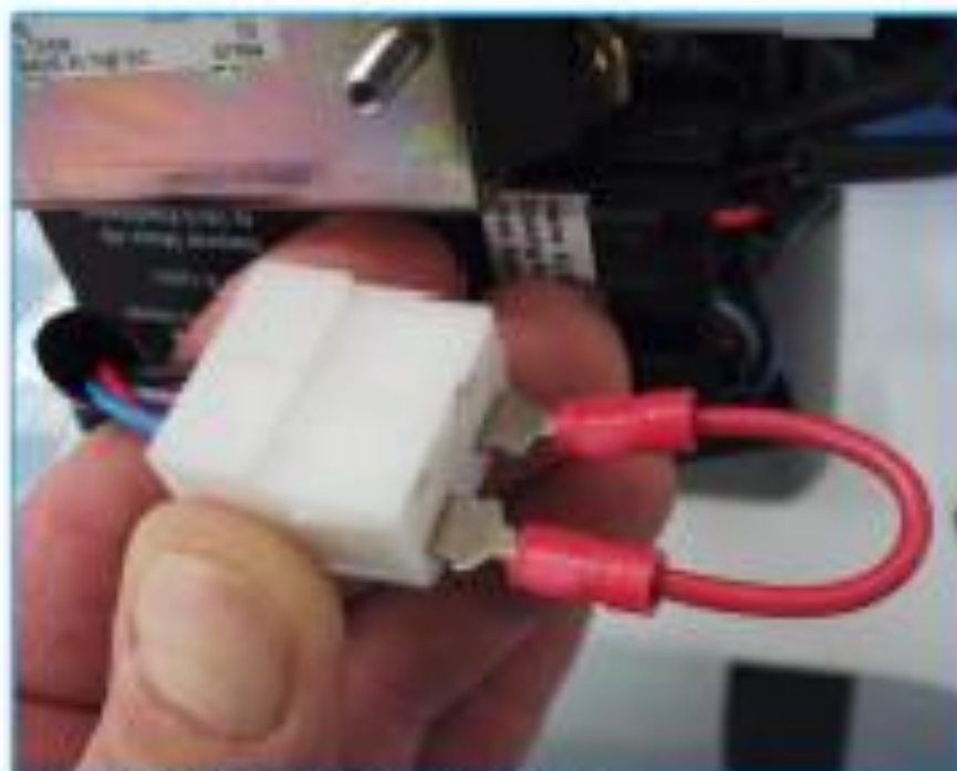
Jumping red to grey on motor pigtail
