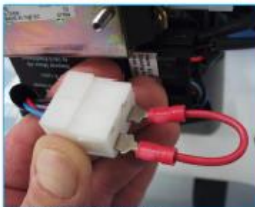
Jumping red to grey on motor pigtail
