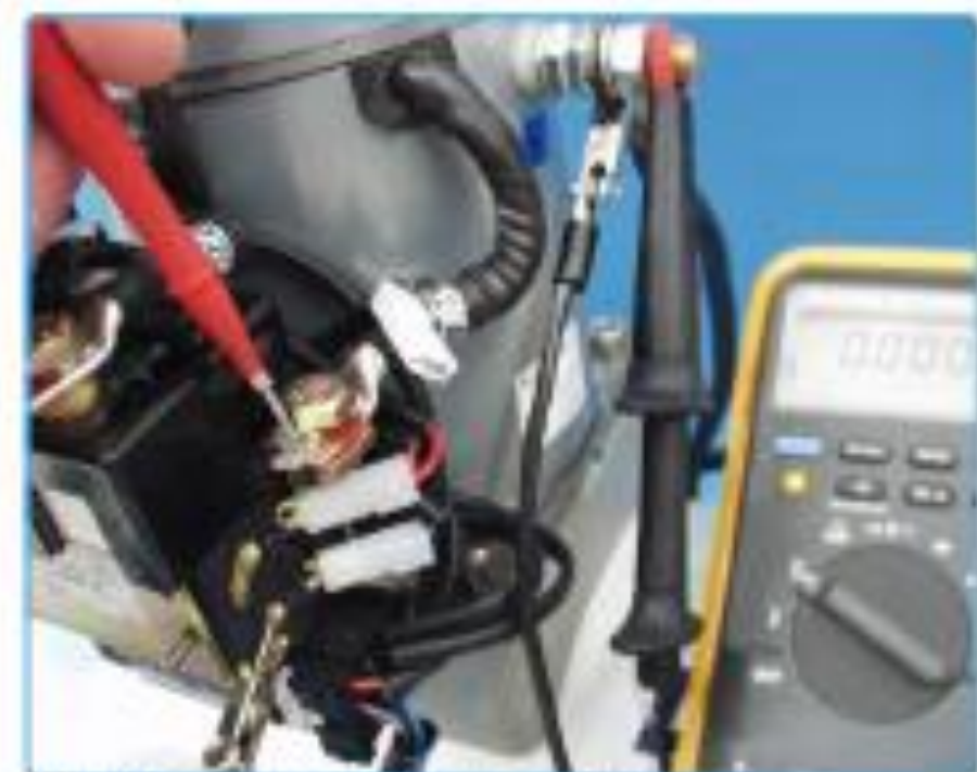
Checking voltage on A2 with ground to blue jumper attached and IPC wire disconnected.
