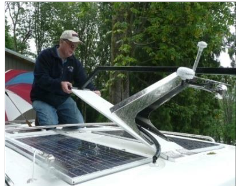
5. Carefully Fold Mast Back
