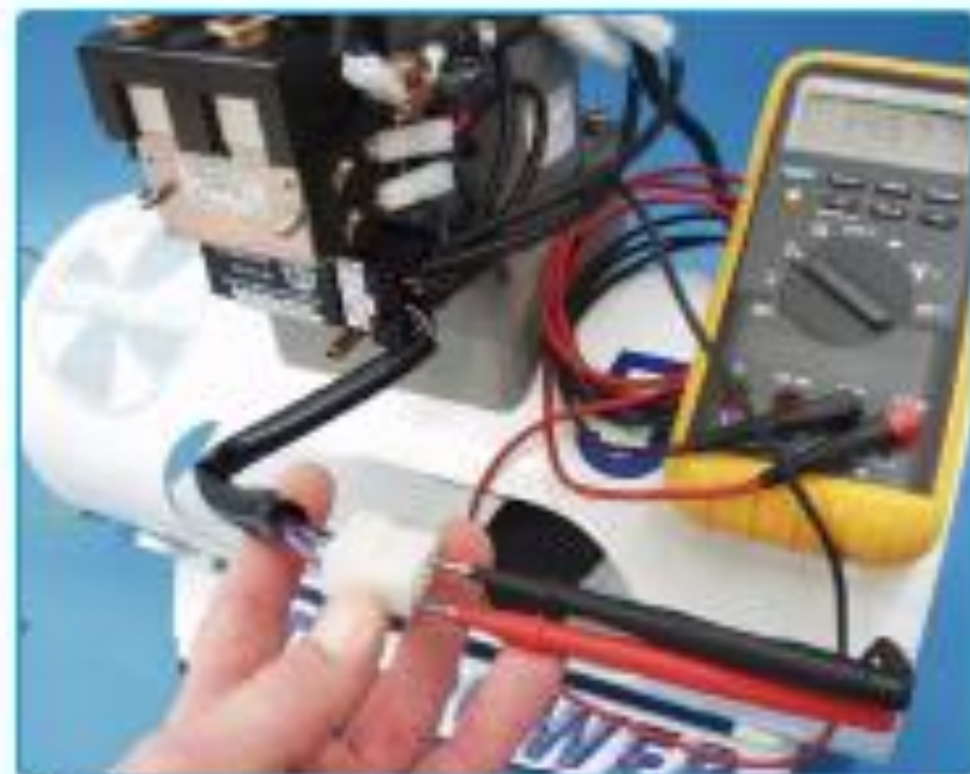
Checking voltage on motor harness
