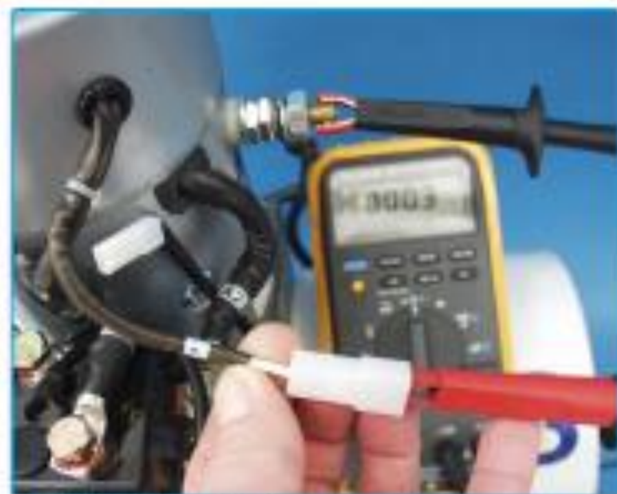
Checking continuity between negative lead and battery negative post
