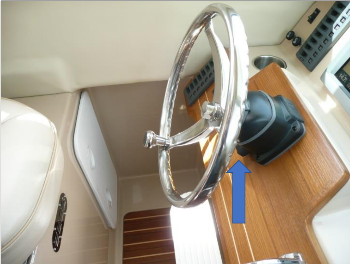
The Tilt Helm lever is located under the steering wheel.
