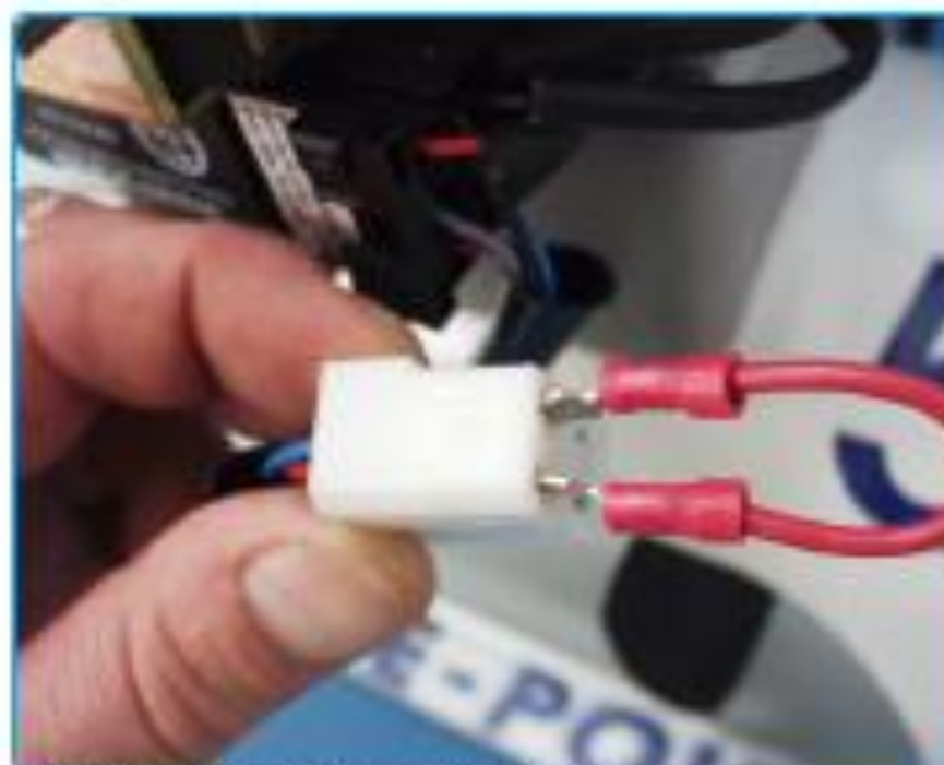
Jumping red to blue on motor pigtail
