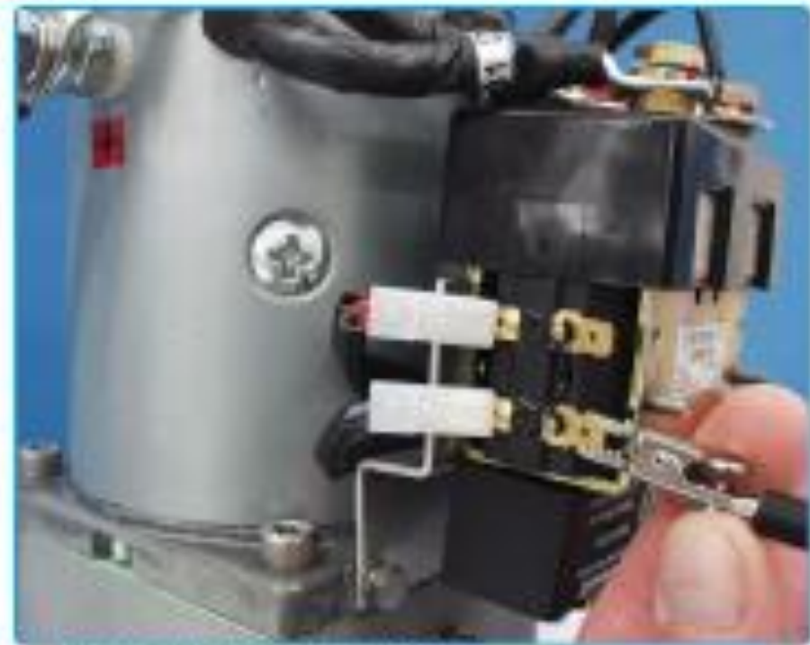
Jumping ground to grey on D1 coil
