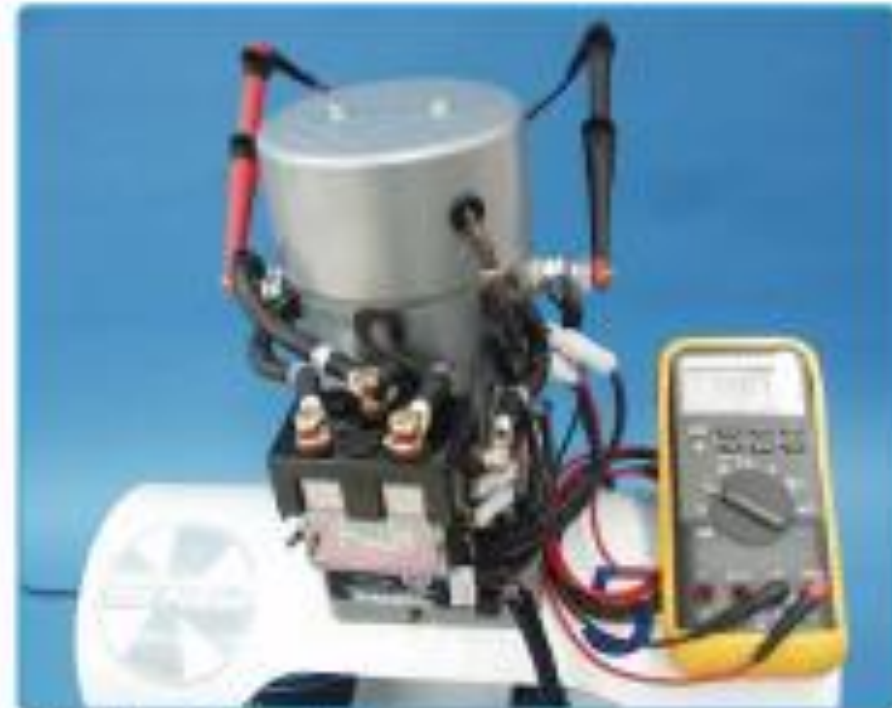
Checking voltage at thruster
