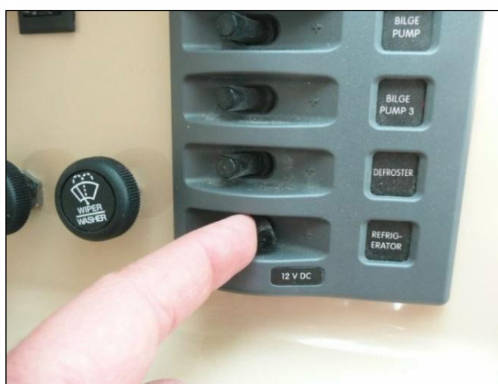
Switch on refrigerator, Lower left DC panel
