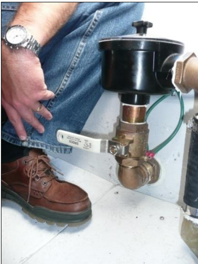
Engine Cooling Water Ball Valve OFF
