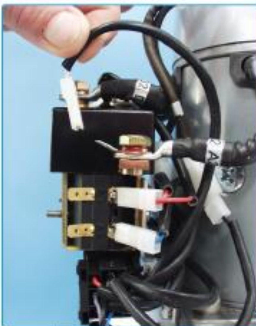
Disconnecting white IPC sensor wire
