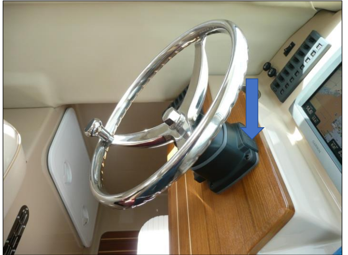
The hydraulic fluid (Teliflex) fills at the top under rubber cover.
