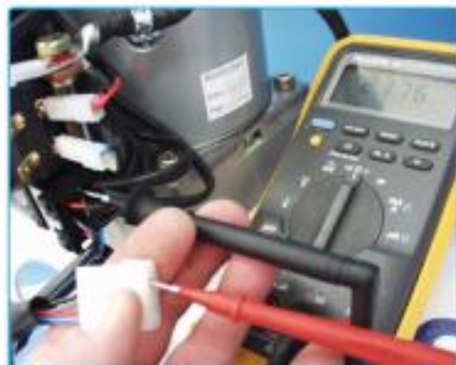
Checking continuity between black in motor pigtail and control box plug
