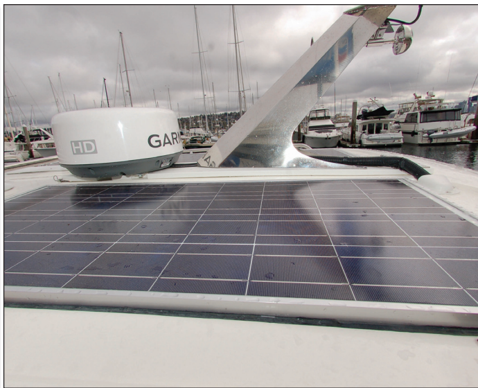
An array of solar panels on the cabin top eliminate the need for a generator.
