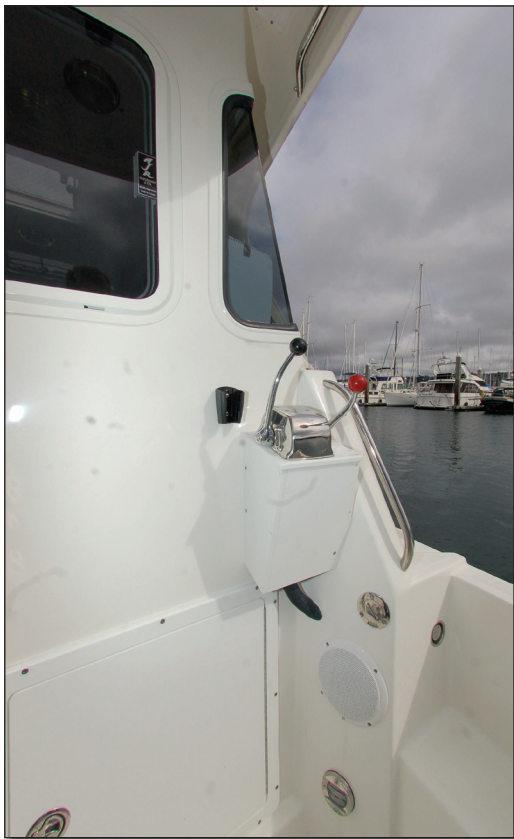
An optional aft station allows control from the cockpit when docking or fishing.
