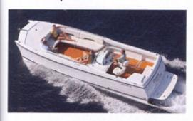
we say Here's evidence that killer efficiency is possible with an internal combustion engine pushing 26 feet of boat. Powered by a single 110 hp Yanmar diesel inboard, the displacement-hulled Aspen 26 burned 5.8 gph at 25 mph, netting a superthrifty 4.3 mpg. At slower speeds, it sips so little fuel that our test gear couldn't record it
