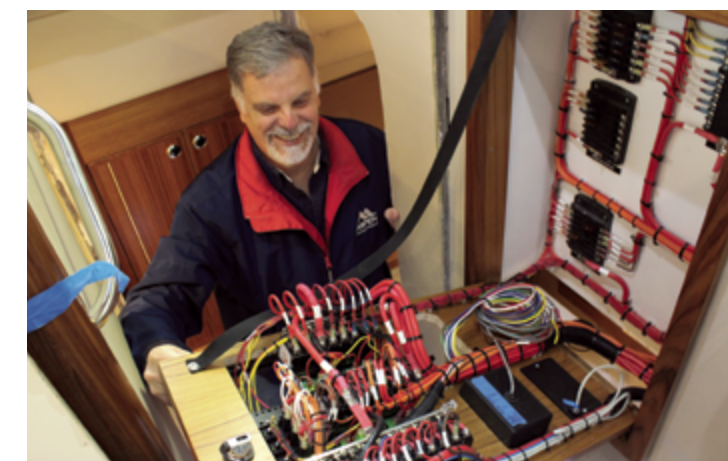
Larry Graf shows off the electrical wiring systems of an Aspen 40 being built at the Burlington factory at the time of this writing. The king-size berth of the master stateroom is around the corner to his left.
