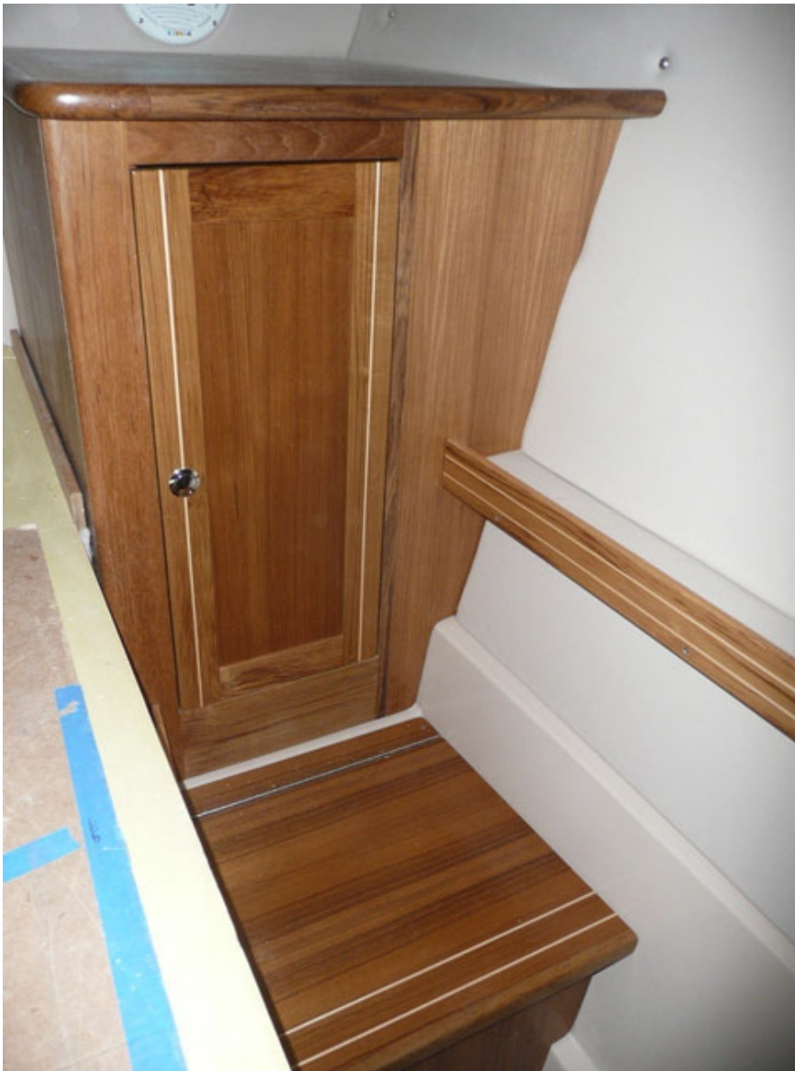
Hanging Locker - Burmese teak hanging locker with seat/step/clothes hamper in King master. Shelf along hull side.
