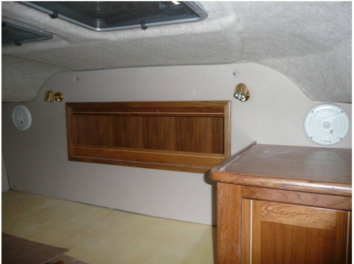
Teak Shelf - Headboard - Teak shelf -- headboard -- with reading lights. Bed lifts for storage under. Bed is made from 4" of premium mattress foam plus a 1" layer of space foam. Let's take a nap!
