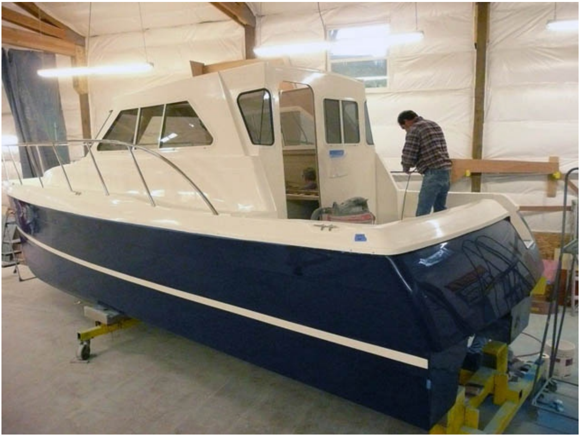
Stern Shot - Note, the swim step is missing; but you can see the transom door cut out.
