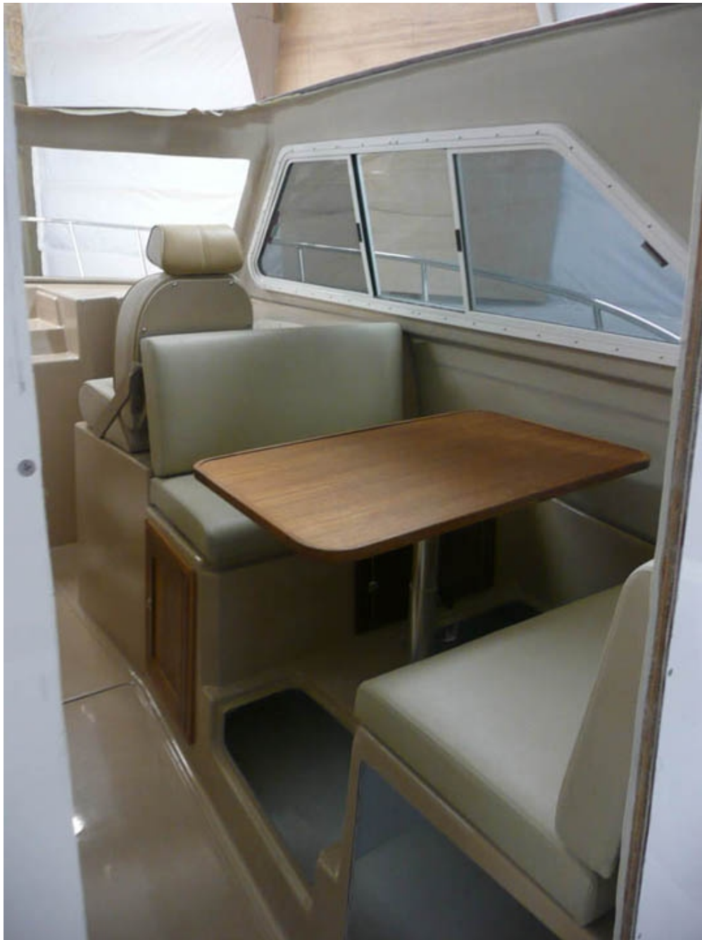
Dinette with Storage Under - Cushions are proto type only, converts to almost a full queen. Note: Slight recess in salon floor, the teak and holly insert flooring fits flush in recess to dress up the look.
