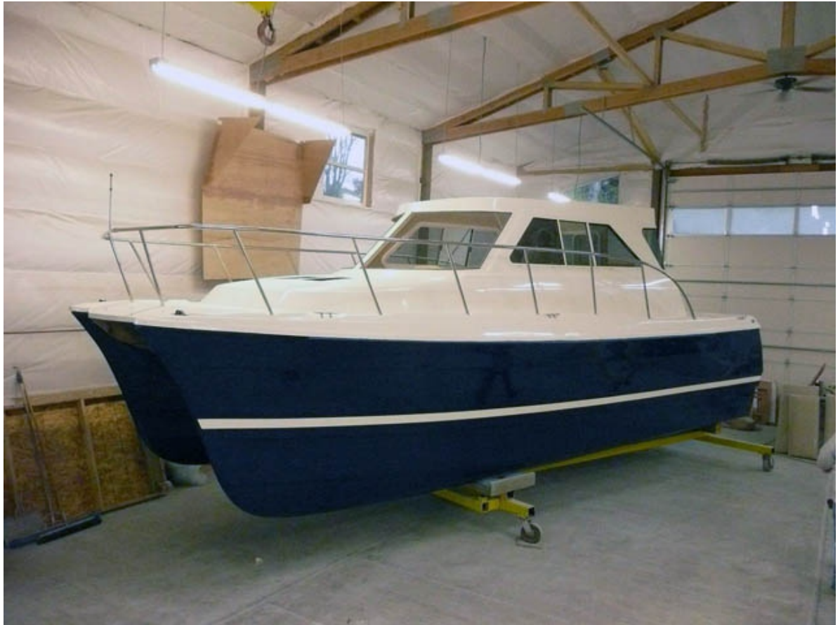
C90 - 28'er Test Fitting of Deck - Missing hardtop & trim components.
