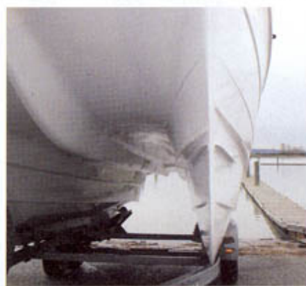
[Above] The Aspen 26 prototype achieves a two-fold increase in fuel efficiency over many vessels its size. [Right] Out of the water, the Aspen cat's unique proa design is easily visible.
