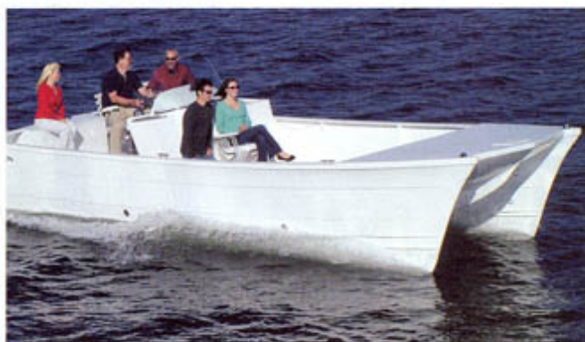
[Above] The Aspen 26 prototype achieves a two-fold increase in fuel efficiency over many vessels its size. [Right] Out of the water, the Aspen cat's unique proa design is easily visible.
